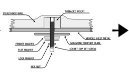
**STEP 8:** Once the Stealthbox® is in place, from the under side of the car. Place the supplied mounting support plate, fender washer, flat washer, lock washer and hex nut onto the exposed Socket Cup Set Screw.
